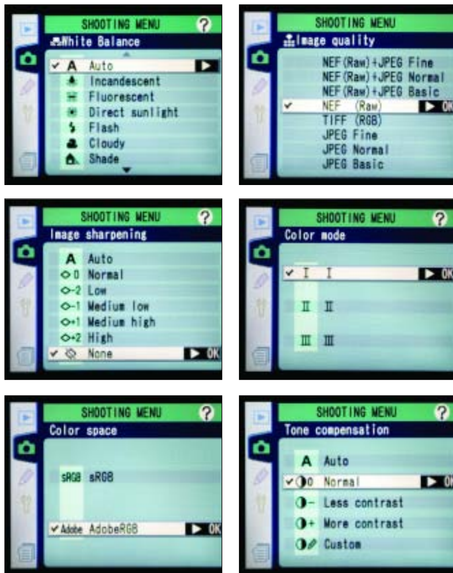
Top left and right—White balance and RAW (quality) settings in the camera menu. Center and bottom rows—Additional capture settings accessed through the menu of the Nikon D2x camera.
